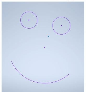
Lock the eyes together, make the center of the arc at the center of the left eye, lock the center of the left eye to the origin, horizontally align the centers of the two circles, and add these dimensions.
